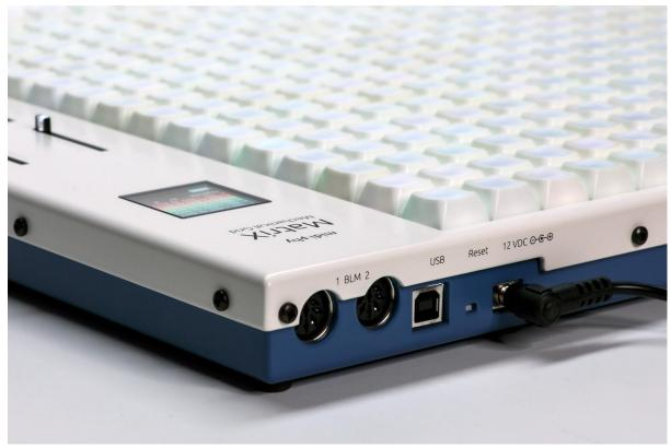
BLM1 and BLM2 are bidirectional MIDI ports that connect to two sequencers, e.g. to a midiphy SEQ v4+ and/or LoopA. Press the dedicated button (↔) to switch between these ports and control the connected device at any time.
